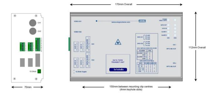
The **AMG5513A6B9** is a standalone transmit unit designed to transmit & receive 1 data signal, 1 Bi-directional alarms plus 1 Echelon FTT10A data channel plus 1 Bi-directional audio channel over one Singlemode optical fibre.
